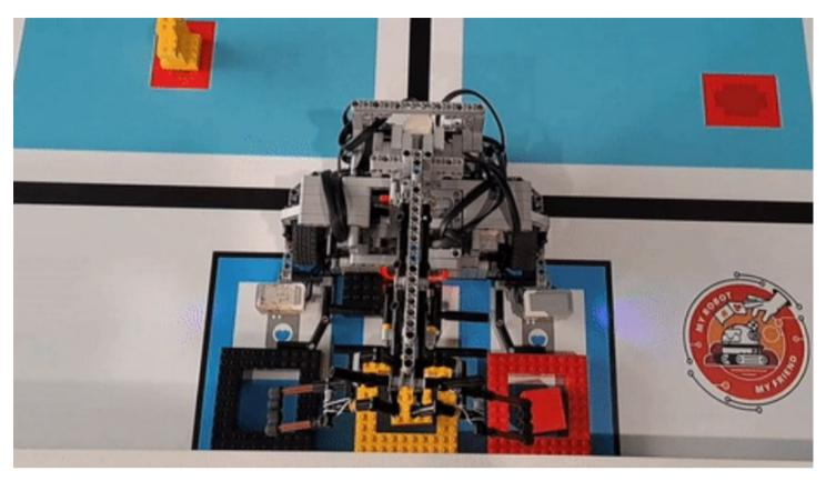
For physical alignment, we realign the robot against the wall before each laundry deposit to 'reset' the errors accumulated in heading and position, increasing reliability.
