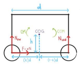
The robot is travelling to the left. When the robot decelerates, there is a maximum decelerating force,  $F = \mu N$  where  $\mu$  is the coefficient of friction and N is the normal force.
