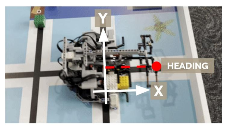
Line intersections are used before each room and the laundry area, aligning the robot in 3 axes.
