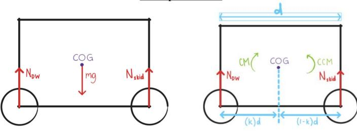
$N_{DW}$  is the normal force acting on the driving wheel.  $N_{skid}$  is the normal force acting on the skid wheel.
