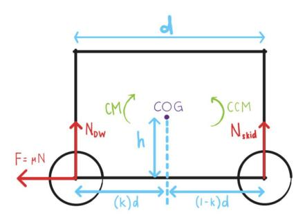
When the robot decelerates, there is a maximum accelerating force,  $F = \mu N$  where  $\mu$  is the coefficient of friction and N is the normal force.
