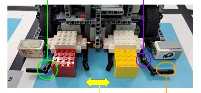
Storage areas spaced to collect both water bottles simultaneously
